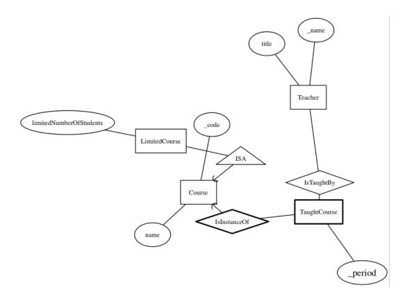
The natural language descriptions on the left are mechanically generated from the E-R model component descriptions on the right. The graphical diagram is generated from the same descriptions. The descriptions thus have a formal notation, which was created *ad hoc* for the Query Converter (qconv) tool, and which supports the generation of both natural language and of graphical E-R diagrams.
